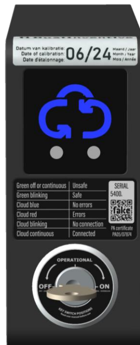
Figure 9 Manually switched 'OFF'
