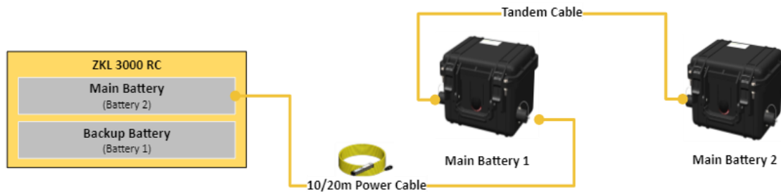
Figure 6 ZKL 3000 RC & Tandem Main Battery Configuration
