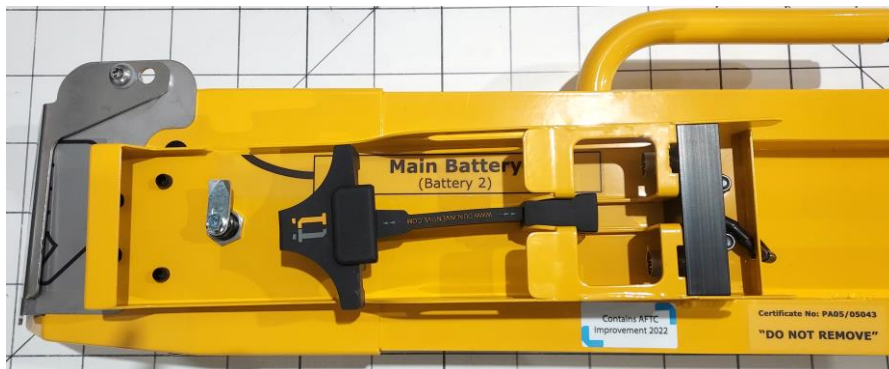
Figure 3 ZKL 3000 RC Battery Connections
