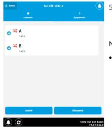
5. Tap "On" or "Off" to switch the rail devices in the selected protection zones On or Off respectively.
